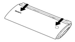
**3.** Aline a SIM card with the mark above the slot, and then carefully slide the SIM card into the slot until it clicks into place.
